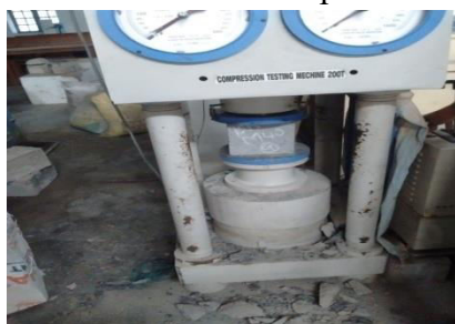
Cube compressive strength test
